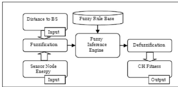
Fig.1. Block Diagram of Fuzzy Logic Control [8]
